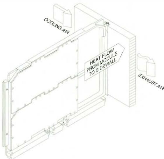
Figure 6 Thermal Flow to the Heat Exchanger
