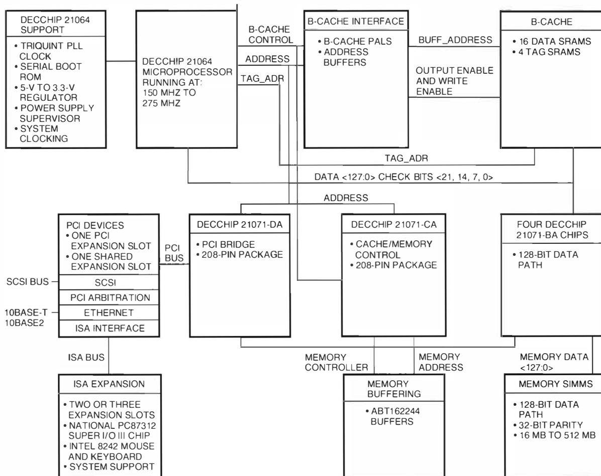
Figure 2 Block Diagram of the EB64+ Module
