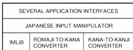
Figure 9 HM Component Structure
