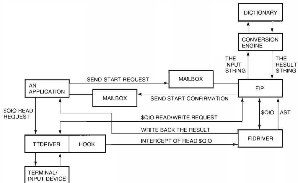
Figure 10 FIP Environment for Manipulation of Japanese Input
