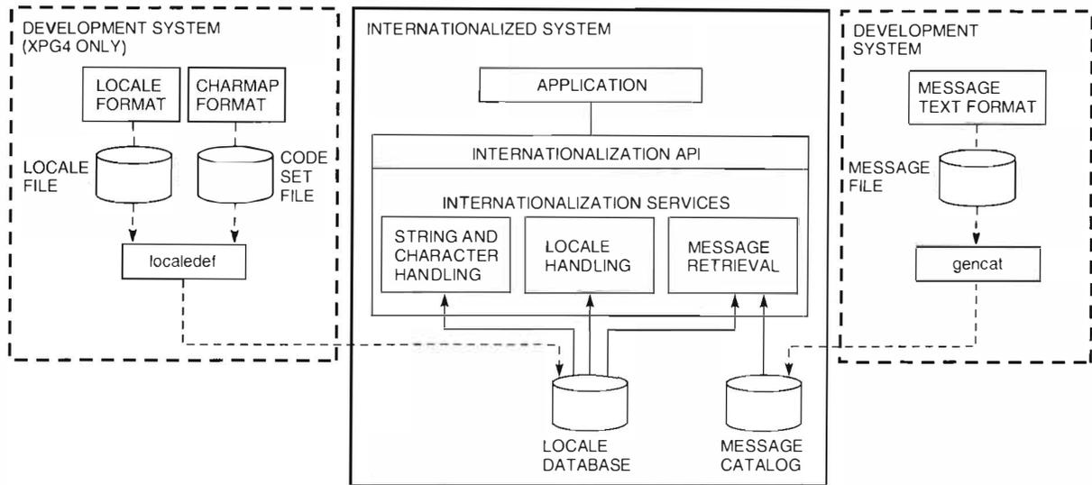
Figure 1 Components of the X/Open Internationalization Model
