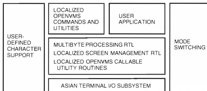
Figure 4 Asian OpenVMS System Structure
