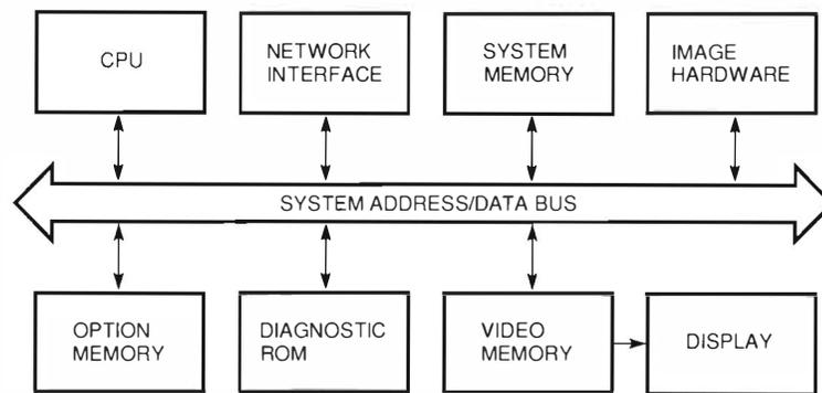
Figure 3 VT1200 System Architecture
