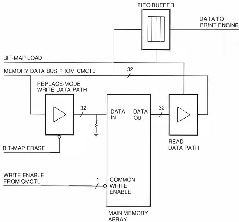
Figure 3 Scan-erase Circuit
