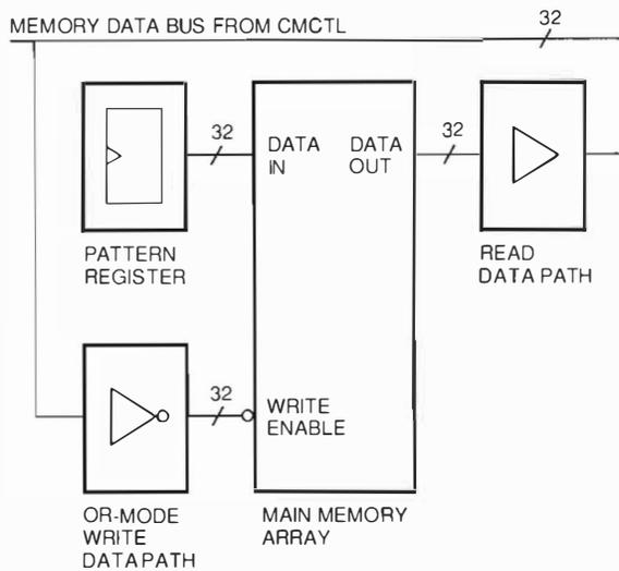
Figure 2 OR-mode Circuit
