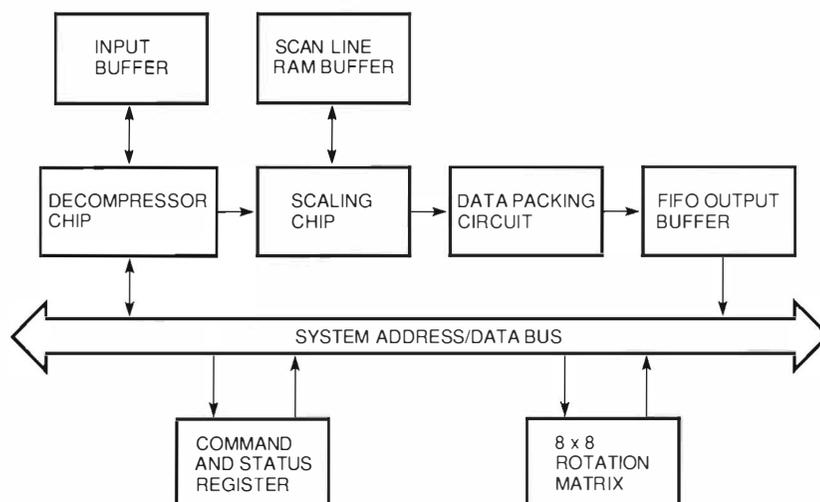
Figure 4 Block Diagram of DECimage 1200 Accelerator Hardware
