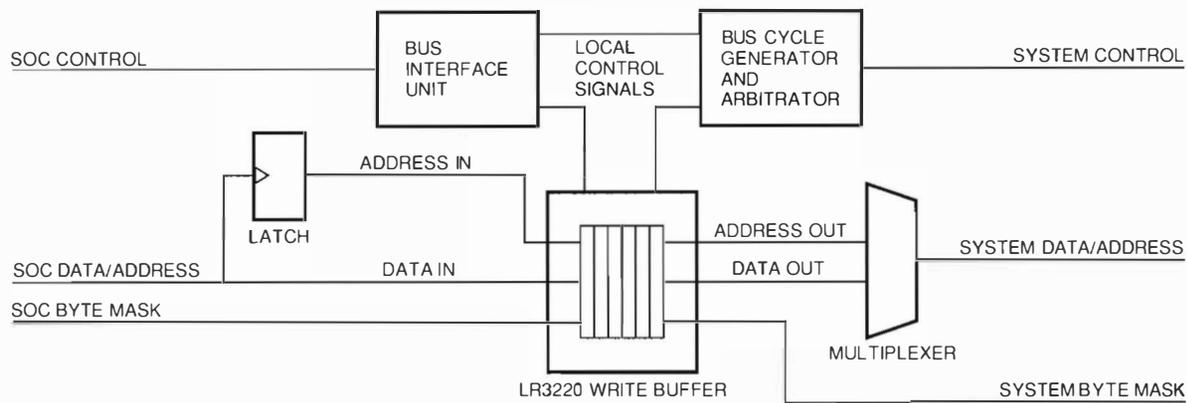
Figure 5 Write Buffer
