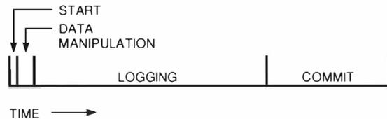
Figure 3 Profile of a Transaction Modifying One Record
