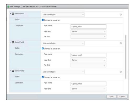
The two figures below show how to set up pipes between two local virtual machines where one plays the role of VMS console. This could be a virtual machine guest running any OS that supports a terminal emulator.
