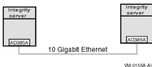
Figure 4.2. Point-to-Point 10 Gigabit Ethernet OpenVMS Cluster
